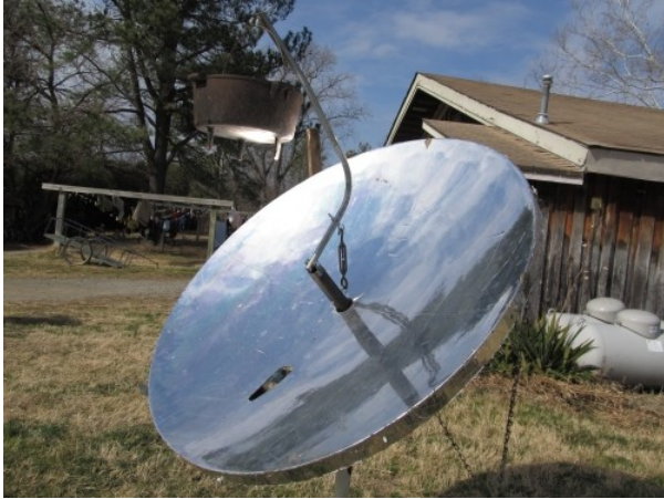
Living Energy Farm's parabolic solar cooker, which uses a simple two chain adjustment mechanism.
