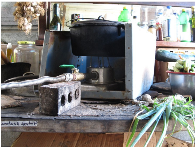
Our homemade burner built from an aluminum pot and some long bolts.
