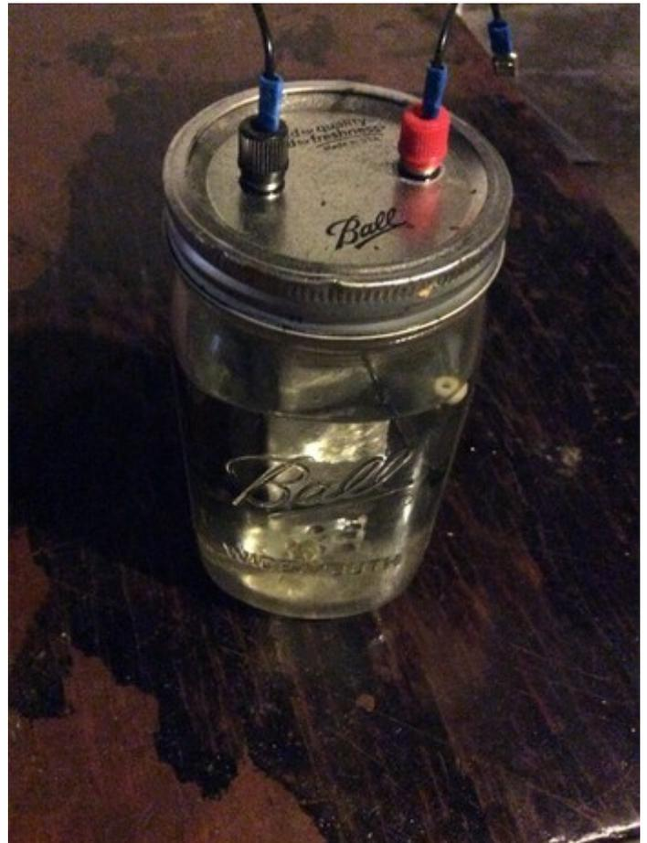
*Prototype NiFe battery. Cheap, durable, homemade? We hope so.*
